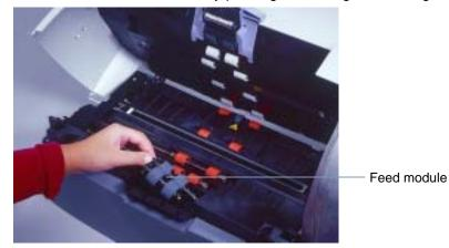
3. Manually rotate and wipe the feed module rollers with a roller cleaning pad.
